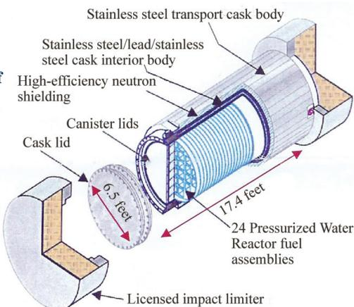
Right: diagram of transport cask with canister.
